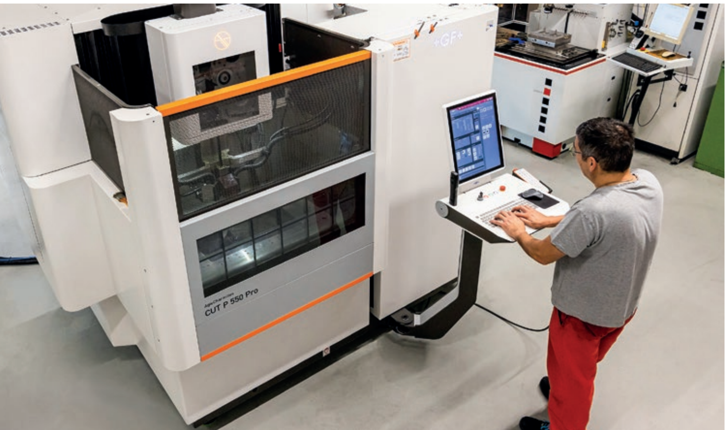
The new wire eroding machine for the high-precision production of metallic tools and complex moulds.
